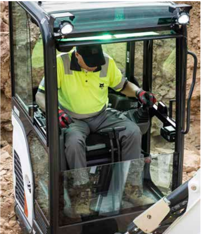
TOPS / ROPS cab with heater
