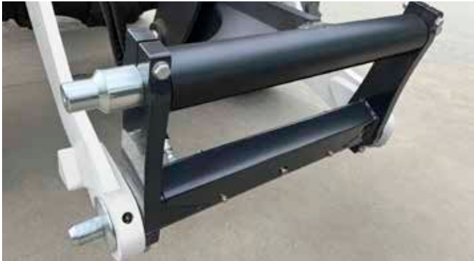
Quick-Tach™ coupler (installed as standard)
