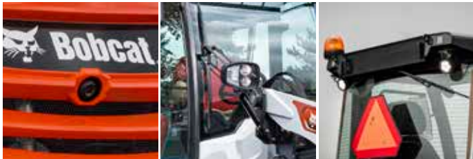
Rear-view camera Road lights LED Work lights LED
